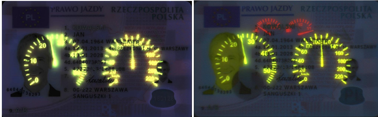
Figure 14: Example of different design motifs visible under different UV wavelengths. On the front side of the Polish driving license, additional instruments become visible at 313 nm UV illumination (right) compared to standard 365 nm UV (left).
