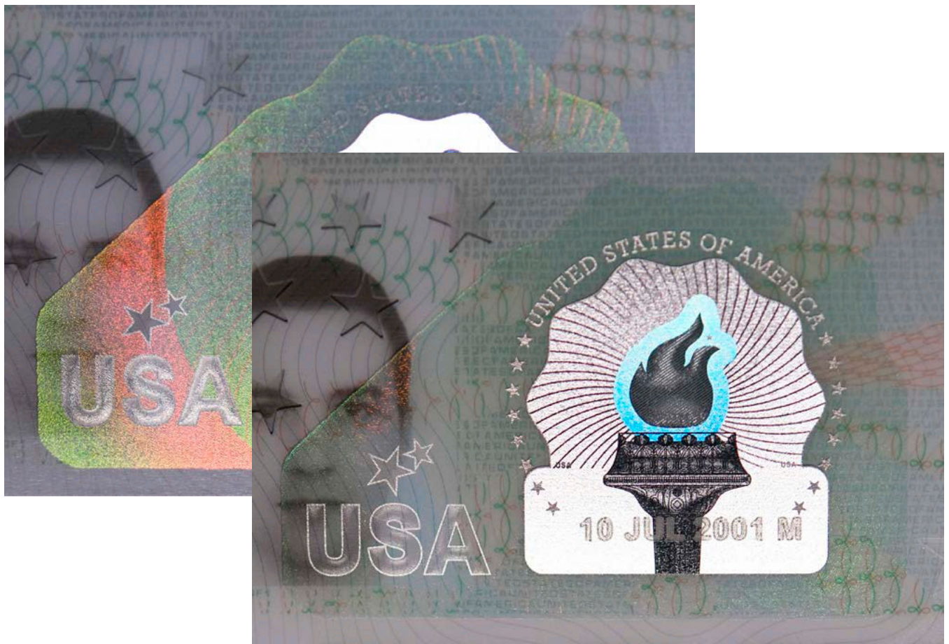
Figure 5: Example of a transparent portion of a DOVID overlapping the portrait. U.S. Permanent Resident Card.
