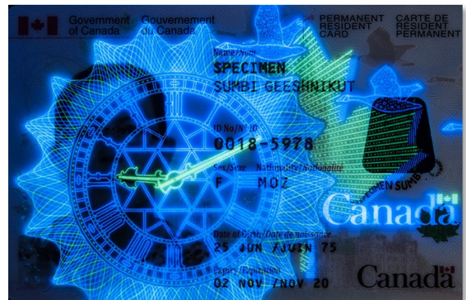
Figure 13: Repeated image (PR card clock) in visible, DOVID, Embossing, UV (Canadian PRC)
