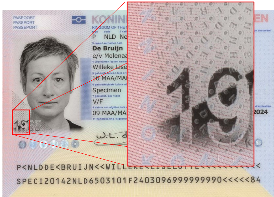
Figure 6: Example of static microprint tactile feature (Dutch passport).
