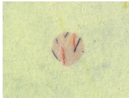
Figure 9: A planchette containing security fibers (Credit: KEESING TECHNOLOGIES)
