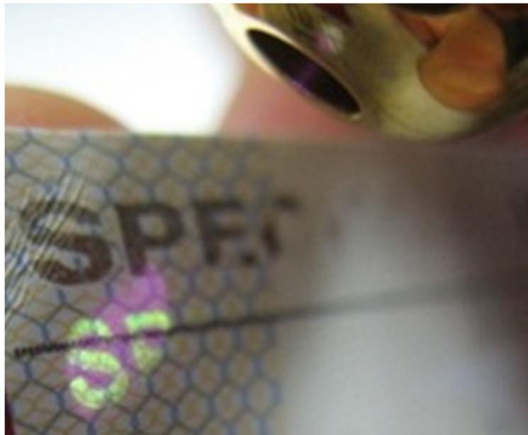
Figure 15: Anti-Stokes (IR fluorescing) print (Credit: Thales)
