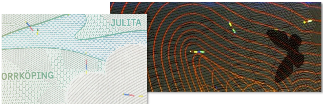
Figure 24: Candy cane fibers in visible and UV
